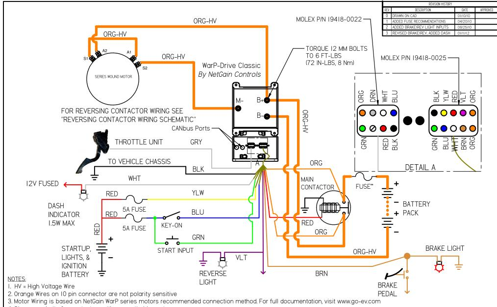
4. Observe polarity for contactors with magnetic blowouts
